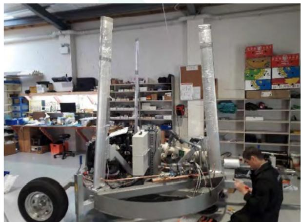
Re purposed Subaru Engines are sourced through Mark at Subwrecks and The Flamingbodyshop in Mahana Rd brings them up like new ready for Collins Automotive to do the electrical wiring. Monteith & Parker supplied new alloy radiators and Wholesale and Industrial across the road add the hoses and clamps.
